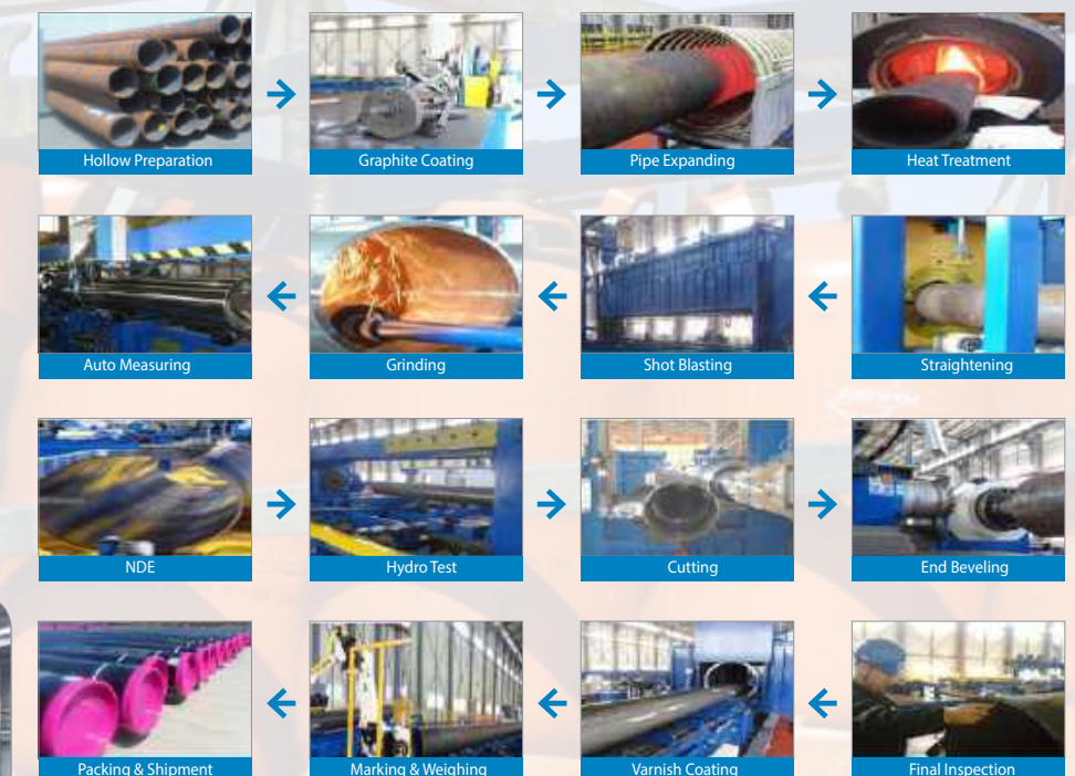
PIPE EXPANDING PROCESS
